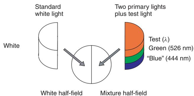
**Fig. 3** Maxwell's method of color matching. A monochromatic test field of wavelength,  $\lambda$ , replaces the primary light to which it is most similar, and a match is made to the white standard by adjusting the intensities of the two remaining primaries and the test field
