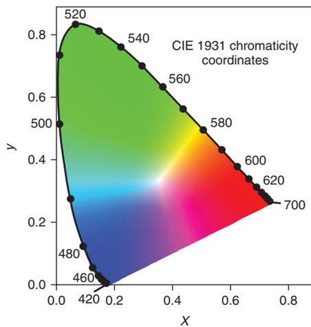
**Fig. 7** CIE (1931)  $x, y$  chromaticity space showing the spectrum locus (continuous line) and spectral wavelengths at every 10 nm (filled circles). A representation of the color of each coordinate is shown, which is necessarily *very* approximate, since it is impossible to reproduce spectral lights in print
