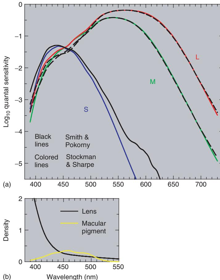
**Fig. 5** (a) S-, M-, and L-cone spectral sensitivity estimates of Stockman & Sharpe [32] (colored lines) compared with the estimates of Smith & Pokorny [29] (dashed lines). (b) shows the lens pigment optical density spectrum (black line) and the macular pigment optical density spectrum (yellow line) from Stockman and Sharpe [32]. Note the logarithmic vertical scale – commonly used in such plots to emphasize small sensitivities
