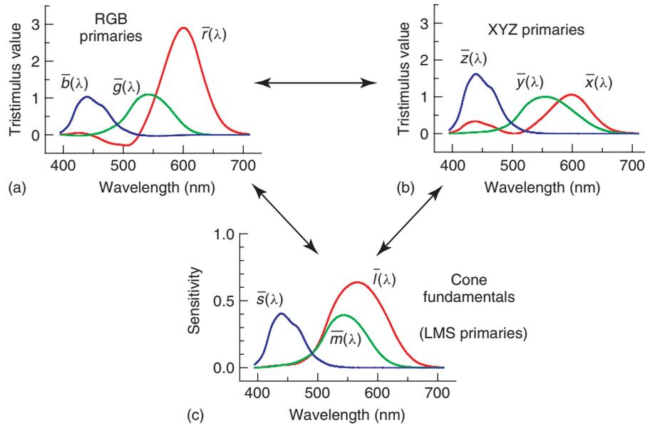
**Fig. 4** CMFs can be linearly transformed from one set of primaries to another. Illustrated here are CMFs (a) for **R**, **G**, and **B** primaries; (b) for the imaginary **X**, **Y**, and **Z** primaries; and (c) for the cone fundamental **L**, **M**, and **S** primaries (bottom). The CMFs are Judd–Vos modified CIE 1931 functions (see Sect. 5.2) and the Smith–Pokorny cone fundamentals (see Sect. 2)
