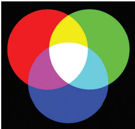
**Fig. 1** Additive color mixing. Simulated overlap of projected red, green and blue lights. The additive combination of red and green is seen as yellow, red and blue as purple, green and blue as cyan, and red, green and blue as white
